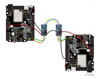
Metro V<sub>HI</sub> to Transceiver VCC Metro IO5 to Transceiver TX Metro IO6 to Transceiver RX Metro GND to Transceiver GND Make the following connections between the two transceivers:
