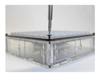
Install four corner screws through both top waffles and into the standoffs.
