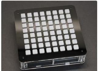
Install the clear top "waffle" piece. Since you'll still be holding the Trellis down, start from one edge, aligning the notches with the tabs on the side pieces, and swing this down into place as you remove your other hand.
