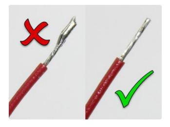
When tinning stranded wires (to prevent fraying and shorts), use just a tiny bit of solder, and make sure it fully flows into the strands. Sometimes you'll want to clip off the very tip of the wire if the iron left a glop or spike there.
