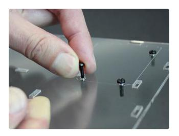
Turn the base over and install three screws in the Arduino footprint area.
