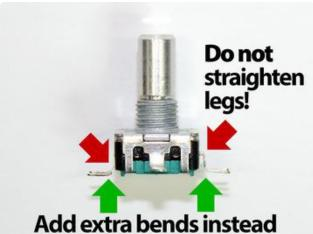
If using rotary encoders, we have the opposite problem when fitting in the case: rather than bending the legs back, we need to splay them outward.
