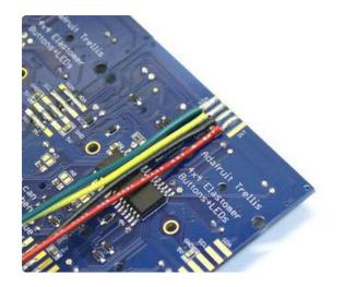
Try pointing the wires "inward" rather than off the edge of the board. This makes it easier to fit in the case.
