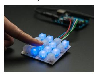
UNTZtrument is based on Adafruit's Trellis, a 4x4 backlit keypad kit.
