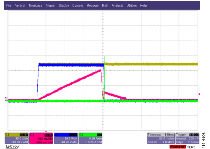
Figure 8. Timer Cycle at Power-Up; Test Points Are as Follows: Channel 1 = V_{IN} , Channel 2 = TIMER, Channel 3 = V_{DS} , Channel 4 = System Current
