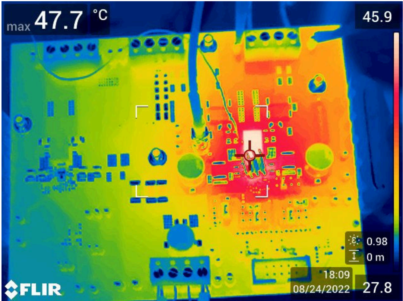
Figure 8-24. Thermal Image at 25°C Ambient
