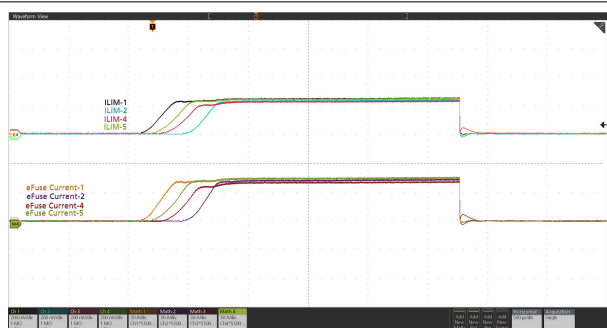
Figure 9-8. Power Up into Short (Current distribution among five devices in parallel): V_{IN} = 12 V, EN/UVLO Stepped Up From 0 V to 3 V, R_{IREF} = 40.2 k \Omega , R_{ILIM} on Each Device = 300 \Omega , and OUT Shorted to GND
