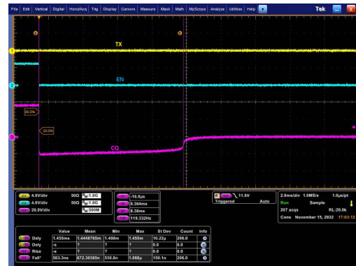
Figure 9-5. CQ in Current Fault Auto Recovery, High Side Mode
