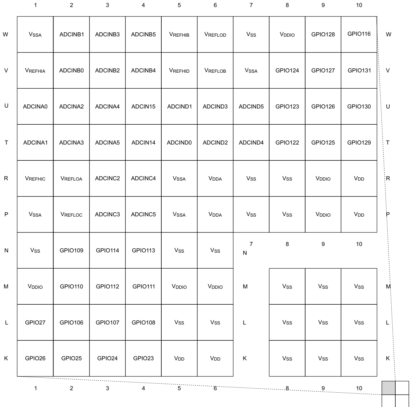
Figure 6-1. 337-Ball ZWT New Fine Pitch Ball Grid Array (Bottom View) – [Quadrant A]
