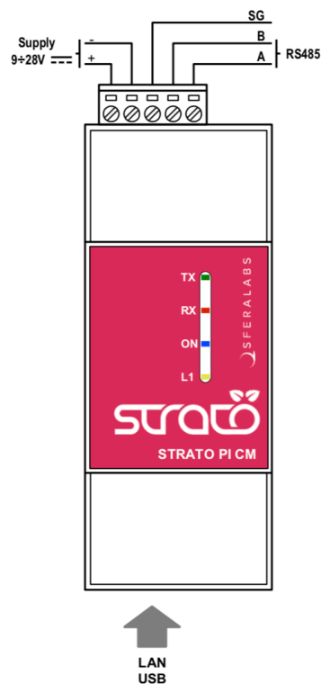
STRATO PI CM CONNECTION DIAGRAM
