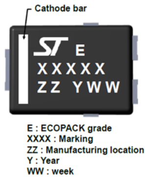
Figure 10. PSMC (TO-277A) marking
