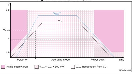
Figure 5. Power-up/down sequence
