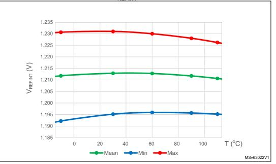
Figure 15. V<sub>REFINT</sub> vs. temperature
