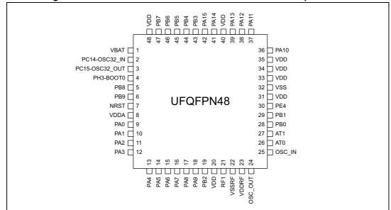
Figure 8. STM32WB50CG and STM32WB30CE UFQFPN48 pinout<sup>(1)(2)</sup>
