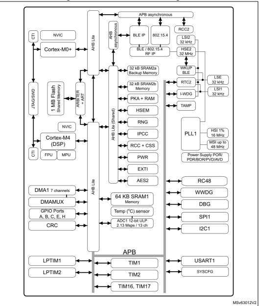
Figure 1. STM32WB50CGxx block diagram
