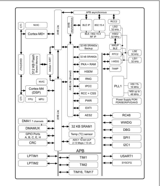
Figure 2. STM32WB30CExx block diagram
