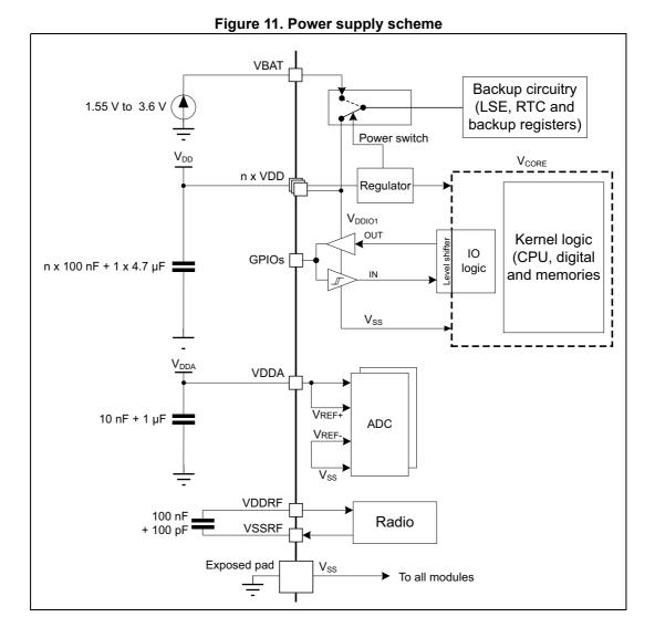
**Caution:** Each power supply pair (such as V<sub>DD</sub> / V<sub>SS</sub>, V<sub>DDA</sub> / V<sub>SS</sub>) must be decoupled with filtering ceramic capacitors as shown in *Figure 11*. These capacitors must be placed as close as possible to (or below) the appropriate pins on the underside of the PCB to ensure the good functionality of the device.
