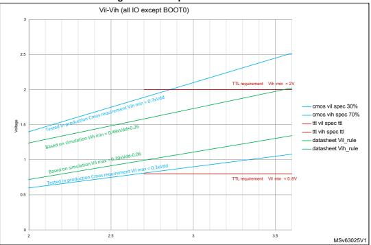
Figure 20. I/O input characteristics
