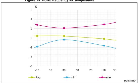
Figure 19. HSI48 frequency vs. temperature
