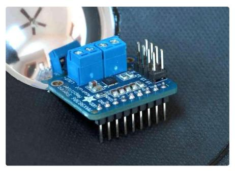
This incredibly small stereo amplifier is surprisingly powerful - able to deliver 2 x 3.7W channels into 3 ohm impedance speakers. Inside the miniature chip is a class D controller, able to run from 2.7V-5.5VDC. Since the amp is a class D, its incredibly efficient (over 90% efficient when driving an  $8\Omega$  speaker at over a Watt).
