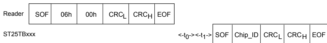
Figure 18. Initiate frame exchange between reader and ST25TB512-AT
