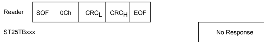
Figure 50. Reset_to_inventory frame exchange between reader and ST25TB512-AT
