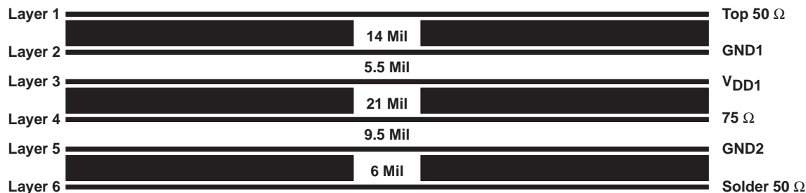
Figure 2–4. TLK2201EVM Layer Construction
