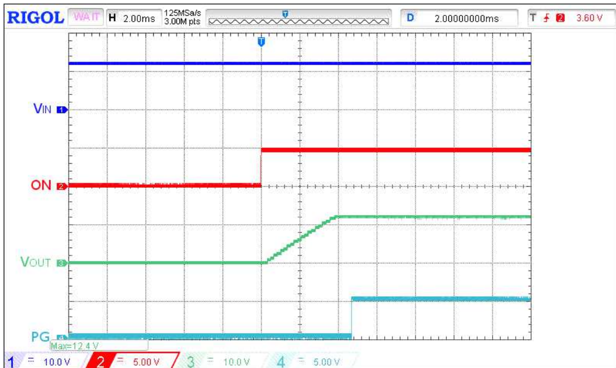
Figure 16. Typical Power Good operation waveform for V_{IN} = 12\text{ V} , C_{LOAD} = 10\text{ }\mu\text{F} , no R_{LOAD}
