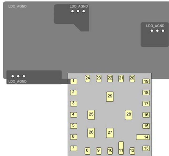
Figure 115: LDO_AGND Layout
