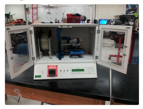
The 3D printer uses a process called fused deposition modeling to construct a solid object from a virtual model. This process involves the controlled deposition of a molten feed stock, typically ABS or PLA plastic, onto a build surface where layer-by-layer the model emerges. Each 3D printer features a series of motors to move the three axis and the extruder, and a controller to move the motors and manage the build process.
