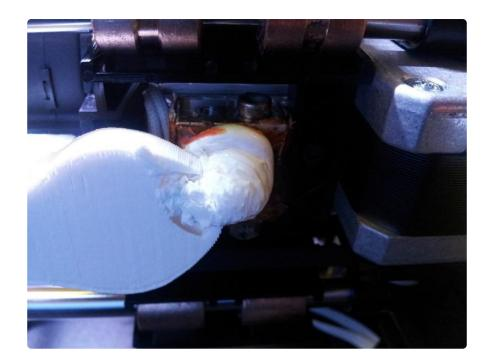
Like any machine, 3D printers should not be left unattended while they are printing. This is especially important with large print jobs as the heat generated by the printing process can cause mechanical failure that, if left unchecked, can cause a fire. Make sure you are familiar with your machine's emergency stop procedure. Most machines feature an emergency stop button (sometimes in the software) to immediately halt the machine. If all else fails, pull the plug!
