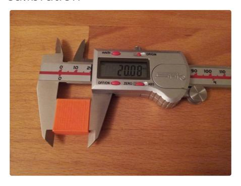
Scale calibration illustrates the process in which you compare the desired dimensions with the actual dimensions your printer produces. The easiest method for accomplishing this is to start by printing a calibration object, like a <u>Calibration Cube</u> () or the <u>Calibration Vector</u> (). Once complete, use a set of calipers to check the dimensions and record your results.
