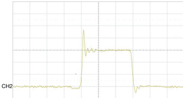
Fig. 17 - Output Switching Waveform CH2 (YLLW) = SW2 (5 V/div.), Time = 10 ns/div.
