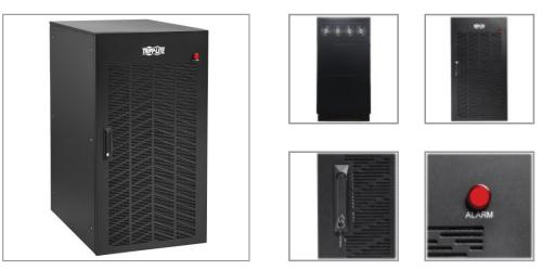
60 kVA/kW transformer provides 600 V (Delta) to 208 V (Wye) step-down and isolation protection to a 3-phase UPS and its load.
