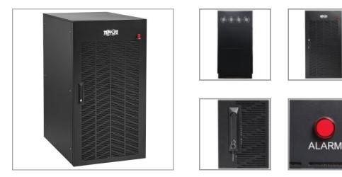
60kVA/kW transformer provides 480V (Delta) to 208V (Wye) step-down and isolation protection to a 3-phase UPS and its load.
