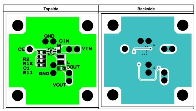
R11 and R12 are arranged as a substitute for R1 so that two resistors can be connected in series.
