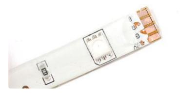
Melt some solder onto the pads to tin them and also burn away any left over rubber.
