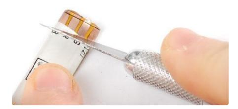
Scrape away the rubber to expose the copper pads.
