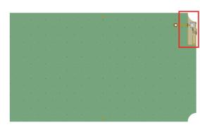
PCB size: 130mm x 75mm x 1mm Antenna area: 16 x 6 mm
