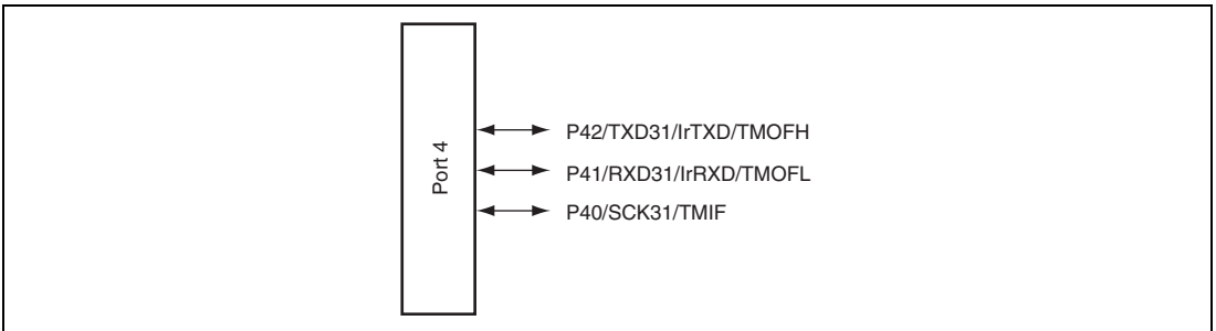
Figure 9.3 Port 4 Pin Configuration
