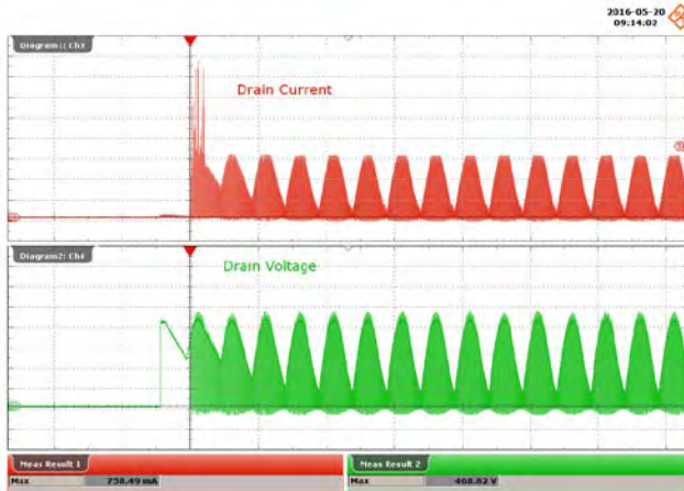
Figure 79 – 300 VAC, 48 V LED Load. Upper: I_{DRAIN} , 100 mA / div. Lower: V_{DRAIN} , 100 V / div., 20 ms / div.
