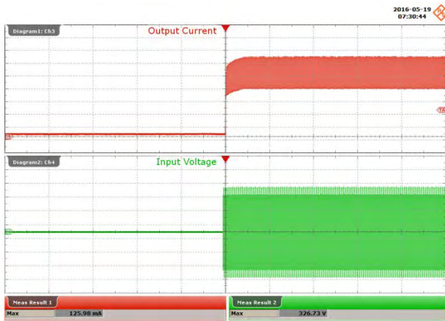
Figure 61 – 230 VAC, 48 V LED, Output Rise. Upper: I_{OUT} , 40 mA / div. Lower: V_{IN} , 100 V / div., 1 s / div.
