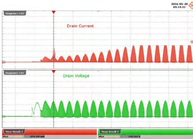
Figure 77 – 90 VAC, 48 V LED Load. Upper: I_{DRAIN} , 100 mA / div. Lower: V_{DRAIN} , 50 V / div., 20 ms / div.
