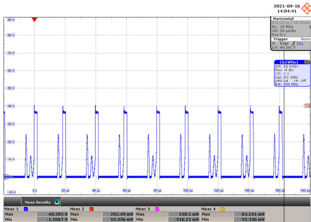
Figure 40 – 5 V SR FET Voltage Waveforms. 265 VAC Input, Full Load. 5 V_{MAX} = 40.39 V . 5 V SRFET V_{MAX} : 10 V / div. 20 \mu s / div.
