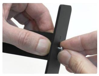
Slots in the leg pieces are "keyed" to fit into the tabs on the cross brace. Position a leg using these tabs and slots, then install a #4-40 1/2" screw through the middle, meeting up with the nut held in the cross brace.
