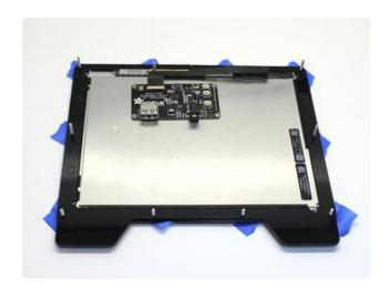
The LCD can now be placed face-down between the corner supports, and all the various protuberances should fit neatly into corresponding cutouts around the perimeter. It may need a little wiggle to make this happen.
