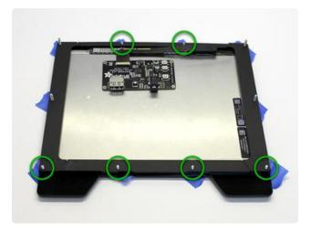
With the edge pieces in place, six nuts can be installed over the shorter (1/2") screws, in the positions marked here. The four longer screws should not receive nuts yet!
