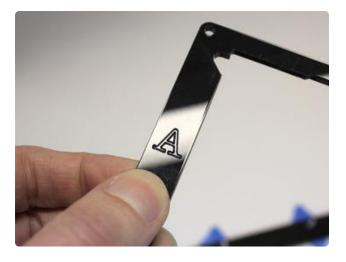
Unlike most of the other parts, the four L-shaped corner supports are all unique and have a very specific orientation. Each is etched with a letter: A, B, C and D.
