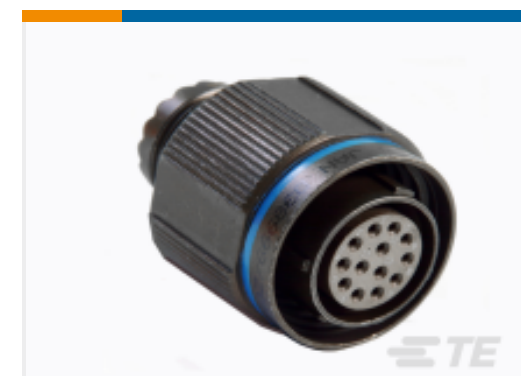
TE Part # YDTS26F15-19PDV001 Straight Plug: D38999, 15-19 Insert, Electroless Nickel Plating
