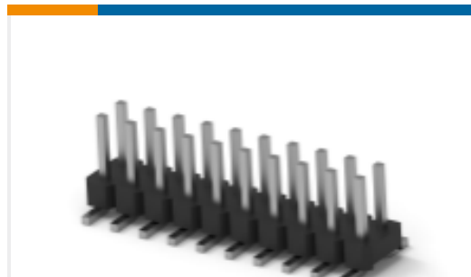
TE Part #1-2842144-0 20P,2MM,BRK HDR,DRV,T,SMD,0.76 AU,TR W/CAP
