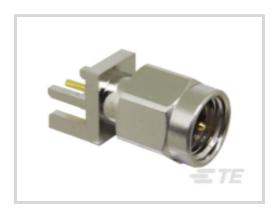
RF Interface: SMA RF Connector Style: Plug Impedance: 50 Ω RF Connector Coupling Mechanism: Threaded Operating Frequency: 0–18 GHz
