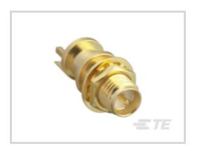
RF Interface: **RP-SMA** RF Connector Style: **Jack** Impedance: **50** Ω RF Connector Coupling Mechanism: **Threaded** Operating Frequency: **0 – 18 GHz**
