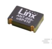
TE Part #L9000152-01 Antenna uSP PCB RPC 410 868MHz SMT T&R
