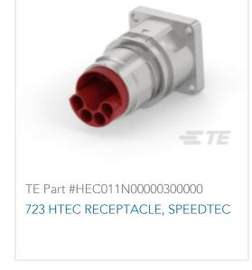
Standard Circular Connectors, Cable-to-Panel, Signal, Panel Mount, Electrodeposited Nickel, Zinc Alloy, PBT GF, Size 15, Shielded, Receptacle
