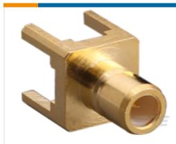
TE Part # CONSMB001-G SMB Jack 50 Ohm PCB Through Hole
