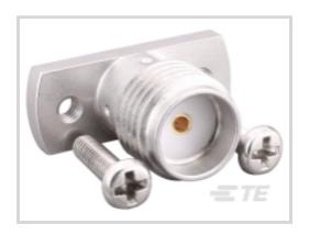
RF Interface: SMA RF Connector Style: Jack Impedance: 50 Ω RF Connector Coupling Mechanism: Threaded Operating Frequency: 27 GHz
