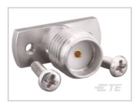
RF Interface: SMA RF Connector Style: Jack Impedance: 50 Ω RF Connector Coupling Mechanism: Threaded Operating Frequency: 27 GHz Features
