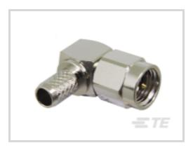
RF Interface: SMA RF Connector Style: Plug Impedance: 50 Ω Compatible With RF Cable Type: RG 141, RG 58 RF Connector Coupling Mechanism: Threaded
