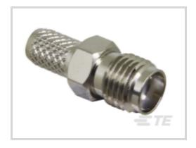
RF Interface: SMA RF Connector Style: Jack Impedance: 50 Ω Compatible With RF Cable Type: RG 141, RG 58 RF Connector Coupling Mechanism: Threaded
