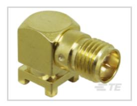
RF Interface: **RP-SMA** RF Connector Style: **Jack** Impedance: **50** Ω RF Connector Coupling Mechanism: **Threaded** Operating Frequency: **12.4 GHz**
