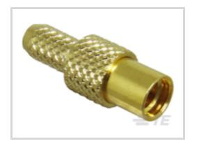
RF Interface: MMCX RF Connector Style: Jack Impedance: 50 Ω Compatible With RF Cable Type: RG 174, RG 188, RG 316 RF Connector Coupling Mechanism: Snap-On
