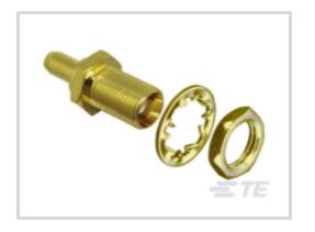
RF Interface: MCX RF Connector Style: Jack Impedance: 50 Ω Compatible With RF Cable Type: RG 178, RG 196 RF Connector Coupling Mechanism: Snap-On
