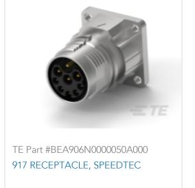
Standard Circular Connectors, Cable-to-Panel, Power & Signal, Panel Mount, Electrodeposited Nickel, Zinc Alloy, PBT GF, Size 23, Shielded, Receptacle
