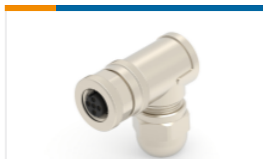
TE Part #T4112412041-000 M12 F, 4P GOLD B_CODE RA SHIELDED PG9
