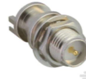
TE Part # L9000254-01 RP-SMA Jack 50 Ohm .031 PCB Edge Mount
