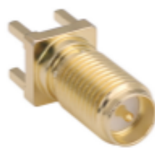
TE Part # CONREVSMA008-G RP-SMA Jack 50 Ohm PCB Through Hole
