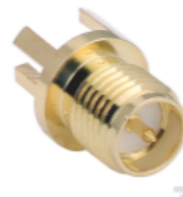
TE Part # L9000251-01 RP-SMA Jack 50 Ohm .062 PCB Edge Mount
