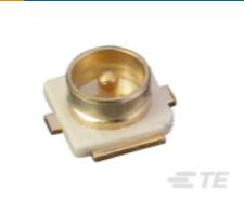
TE Part # CONMHF1-SMD-G-T U.FL/MHF1 Jack 50 Ohm PCB Surface Mount
