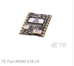
TE Part #RXM-418-LR Module LR 418MHz AM OOK RX RCVR
