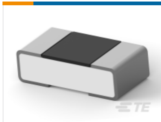
TE Part #6-2176363-9 RQ 0402 2K21 0.1% 10PPM 5K RL
