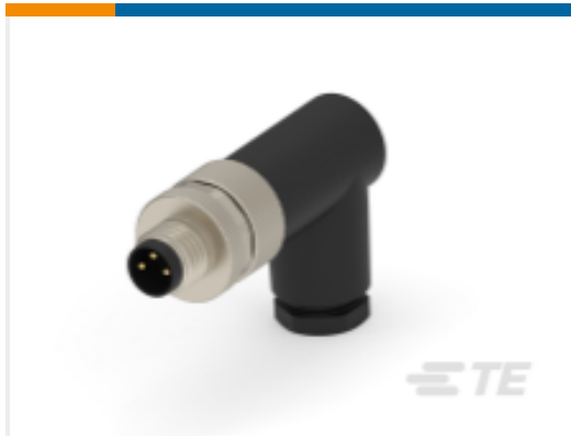
TE Part #T4013008031-000 M8,SCREW, MALE,R/A,UNSHIELD,3P, GOLD
