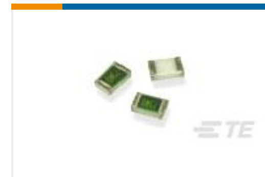
TE Part #1676144-2 RN 0805 102K 0.1% 10PPM 1KRL
