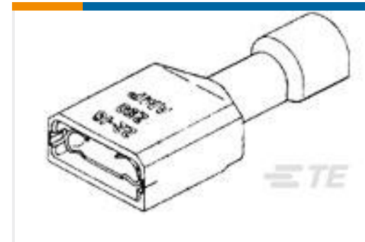
TE Part #3-350820-2 ULTRAFAST 250 ASSY REC 16-14 TPBR LP
