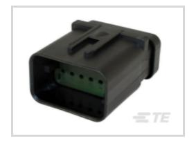
Connector System: Wire-to-Wire Number of Positions: 12 Connector & Housing Type: Housing for Male Terminals Centerline (Pitch): 4.5 mm [.177 in ] Sealable: Yes
